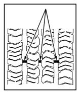
One way to tell when it is time for new tires is to check the treadwear indicators, which appear when your tires have only 1/16 inch (1.6 mm) or less of tread remaining. Some commercial truck tires may not have treadwear indicators. You need new tires if any of the following statements are true:
